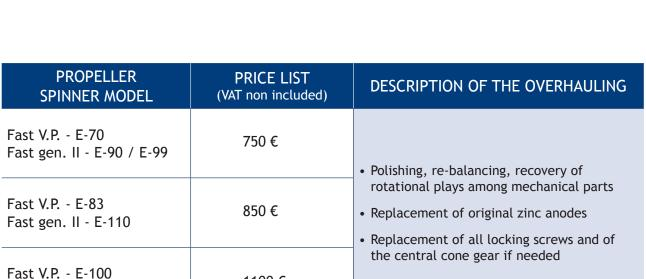
In case the propeller is particularly damaged, MAX PROP®, will send you a detailed free quotation before proceeding with any work.
